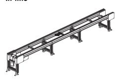
In-line systems are the simplest configuration and form the basis for all other TS4plus configurations.
