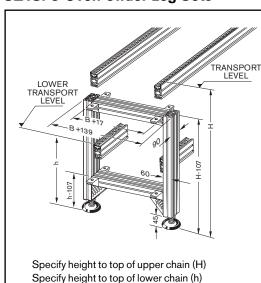
Over/Under leg sets are similar in design to single leg sets, but allow a second line to be installed below the main line, typically as a return line for empty pallets. The height to the top of the lower chain must be at least 300 mm, to allow clearance for drives and returns. Sufficient space must be left between the top and bottom heights to allow for pallet and fixture clearance.
