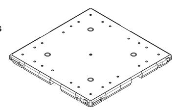
Assembled workpiece pallets also have four pressed-in hardened steel positioning bushings which provide precise location of the workpiece pallet for automated assembly operations when used with Rexroth positioning modules. M8x25 screws (quantities vary according to pallet size) are used to secure the frame modules to the support plates.
