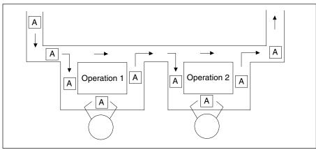
"Cycle-independent stations" can be used to balance assembly operations with differing cycle times.
