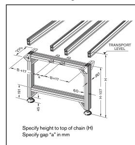
Parallel leg sets are similar to single leg sets, but are used to support two adjacent conveyor sections on a single leg set. To help prevent overloading, each section width (B<sub>wt</sub>) is limited to 843mm.
