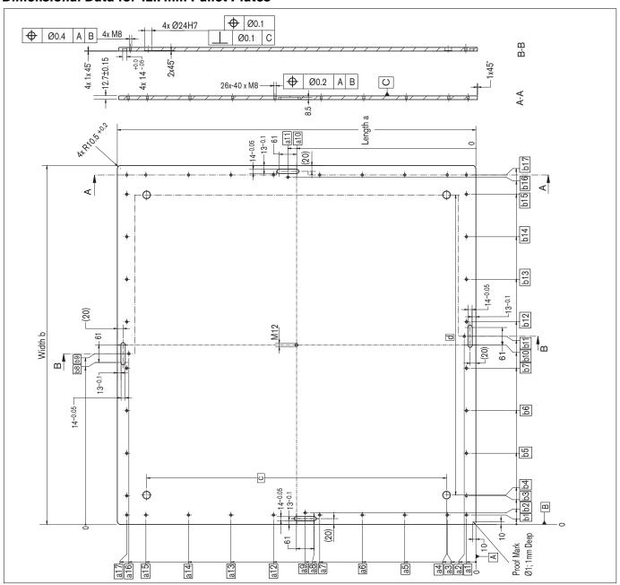
Ordering Information for 12.7 mm Aluminum Workpiece Pallet Plates
