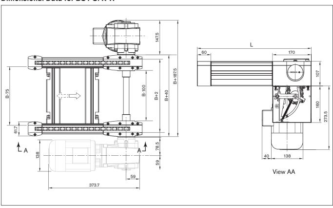
$Transverse\ conveyor\ width\ (B)\ must\ match\ pallet\ length\ (L_{_{WT}})\ or\ width\ (B_{_{WT}}),\ depending\ on\ orientation.$
