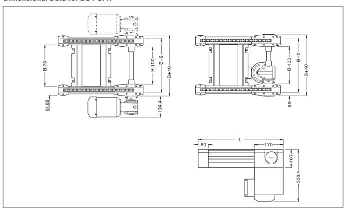
$Transverse\ conveyor\ width\ (B)\ must\ match\ pallet\ length\ (L_{_{WT}})\ or\ width\ (B_{_{WT}}), depending\ on\ orientation.$
