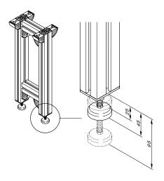
Leg sets must be placed below chain section joints, at maximum conveyor spans of 2000mm and where additional support is needed.
