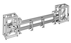
Over/under systems consist of two conveyor sections mounted one above the other. One conveyor section transports the workpiece pallet through the assembly process. The other conveyor section then returns the workpiece pallet to the beginning of the line. The upper and lower sections are connected together by vertical transfer units on each end. Over/under configurations provide a significant savings in floor space requirements, making them ideal for applications where space is at a premium.
