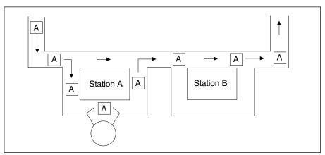
Fluctuations in production quantity can be easily accommodated by bypassing assembly workstations.
