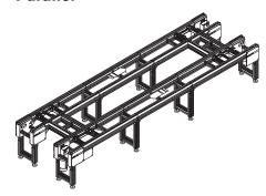
Parallel systems are formed by linking two in-line systems, running in opposite directions, together side-by-side, with track rollers bridging the gap between the lines. Lift Transfer Units move the pallets on and off the main line. This allows continuous circulation of pallets, and can be used where the capacity of a rectangular system is not needed, or where space is
