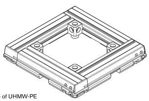
The wear strips are made of UHMW-PE and include an integrated dampening element to absorb the shock when two pallets come into contact with each other.
