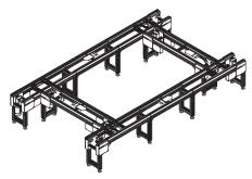
Rectangular systems use in-line conveyors, with Lift Transfer Units at the "corners" to move the pallets on and off the main lines. This layout offers the advantage of continuous pallet circulation without the spacing limitations created by track rollers. In addition, the use of standard conveyor sections for the transverse sections means that there is no loss in load capacity or accumulation capabilities. Process stations can be set up all the way around the conveyor, if needed.
